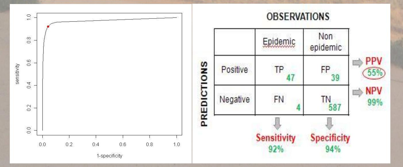
The use of the ROC selected cut-off value (red point) results in poor PPV
